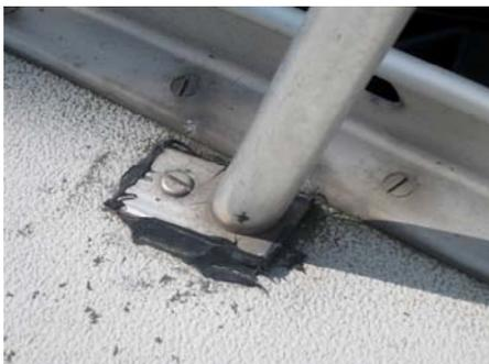
The stanchions are attached to the toerail; each was physically tested and found to be secure apart from those around the port and starboard boarding gates. The forward port gate stanchion was loose and the feet for the aft one did not lie fair to the deck. On the starboard side the foot for the forward gate stanchion has been refastened to the deck, though it still does not lie fair, see photo. The stanchion itself was more secure than the equivalent one on the port side.
